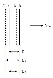
$D_{A}$ ' is the apparent distance of plate A as seen by plate B.  $D_{B}$ ' is the apparent distance of plate B as seen by plate A. Strict application of AST shows that, to a point charge on one capacitor plate
