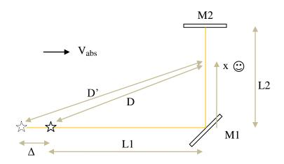
To analyze this problem, we first have to determine the apparent change in position ( $\Delta$ ) of the source as seen from point x, due to absolute motion.
