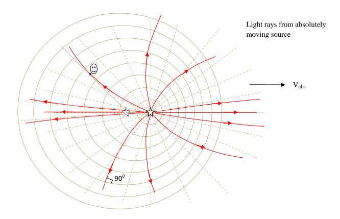
\* note that the above diagram is not drawn accurately. The light rays should always make 90° with the wave fronts. The bending light rays are only for a co-moving observer. For an observer at rest, light rays come as usual in straight lines from the point where they were emitted.
