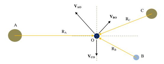
$$V_{abs0} = \frac{M_A}{M_T} V_{AO} + \frac{M_B}{M_T} V_{BO} + \frac{M_C}{M_T} V_{CO} \text{(vector sum)}$$
