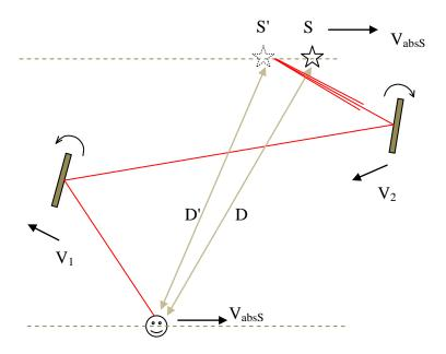
Assume the source emits a very short light pulse just at time t=0. The problem is to determine the time delay of light before it is detected by the observer. This is a complicated problem compared to the Michelson-Morley (MM) experiment in which the light source, the detector, the beam splitter and the mirrors are all at rest relative to each other.
