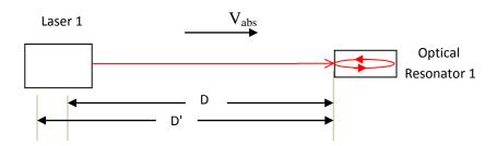
The laser has been represented as a single coherent point source, as shown below.
