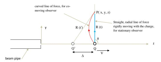
From the figure above, we can see that the maximum transverse electric field is detected at point P when the charge is physically at Q, as measured by the stationary sensor at point P.
