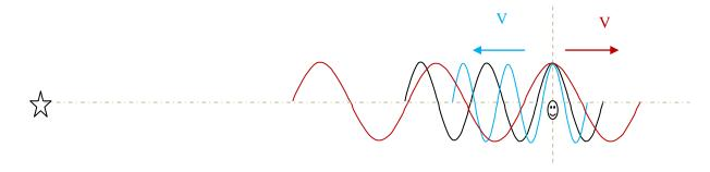
The black wave represents the wave for source and observer at rest relative to each other. The red and blue waves are for the cases of the observer moving away from the source and towards
