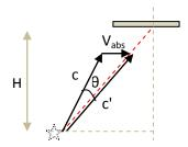
$$\frac{\sin \theta}{V_{abs}} = \frac{\frac{H}{L'}}{c} = \frac{\sin(\theta + \sin^{-1}\left(\frac{H}{L'}\right))}{c'}$$
