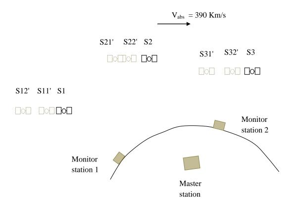
The control stations monitor the satellites from the signals they transmit and send the information to the master station, where the orbit and clock performance of each satellite is computed. These data are then uploaded to each satellite.
