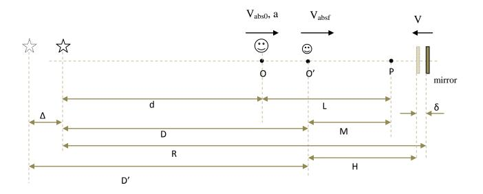
The problem is to determine the time *t* elapsed between emission of light and detection by accelerating observer O of the light reflected from the moving mirror.
