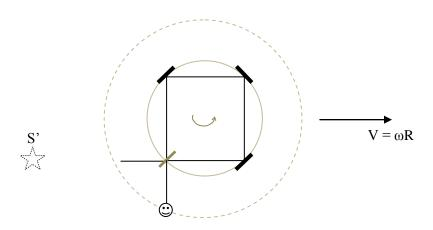
S', which is the apparent point of emission, is at rest, so the speed (group velocity) of light emitted by the source is equal to c in the inertial reference frame in which the device is
