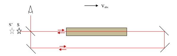
According to Apparent Source Theory, like the Michelson-Morley experiment, the effect of absolute motion is to create only a small fringe shift due to apparent change in position of the source, as seen by the detector.
