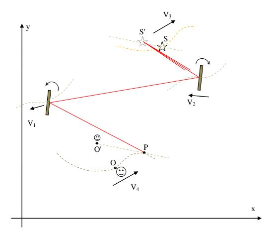
The procedure of analysis is first to define the positions and motions of the mirrors, the beam splitter and other components, the observer, the light source in the absolute reference frame or any convenient inertial reference frame whose absolute velocity is known.
