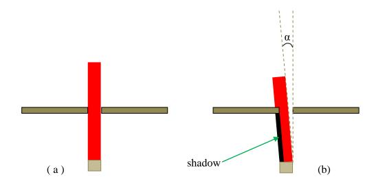
In reality, however, the area of the slit and the area of the sensor may not be equal. In fact, I used a slit width (area) very small compared to the area of the sensor. Moreover, the cross
