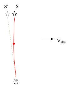
We see that the apparent change in position of the source is due to the curving of the light rays, as shown above. The curve is determined by applying the Apparent Source Theory (AST) at every point. Even though the source is physically, actually at position S relative to the observer, it appears to the observer that it is at position S' and this is due to the curving of the light ray which is a result of absolute velocity.
