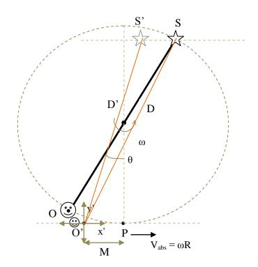
Then the problem is analyzed in the reference frame of O', to get the expression for the time delay of light from emission by the source to detection by the observer O', i.e. the time of flight.
