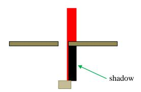
With zero absolute velocity, that the light source should be shifted off the axis of the slit so that it is not completely visible to the sensor. With increase of absolute velocity to the right, more and more light emitting atoms will come into view of the sensor and this may be detected as change in sensor output.
