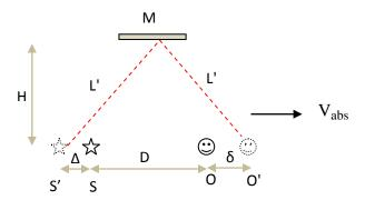
The time T elapsed for the light to travel from S', reflection at mirror, then arrive at O' is equal to the time taken for the observer to move from O to O'. The speed of light is c relative to the apparent source. We have to determine the speed of light c' in the dashed light ray, as seen in the absolute reference frame.
