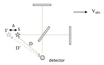
From the above diagram of the Michelson-Morley experiment, arranged for circular or straight parallel fringes, we see that the effect of absolute velocity is just to create an apparent change of the position of the light source relative to the detector, for absolute velocity  $V_{abs}$  directed to the right.
