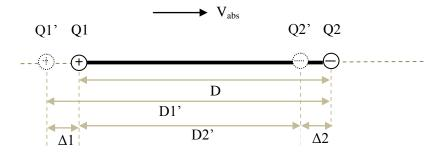
D is the actual, physical distance between real charges Q1 and Q2. D1' is the apparent distance of Q1 as seen by Q2. We can also say that D1' is the distance of apparent charge Q1' from real charge Q2. D2' is the apparent distance of Q2 as seen by Q1. We can also say that D2' is the distance of apparent charge Q2' from real charge Q1.
