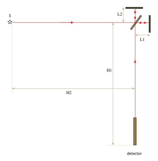
As we have seen above, Apparent Source Theory has revealed the century old mystery of the Michelson-Morley experiment: *increasing the arm length made the apparatus less sensitive to absolute motion*. Moreover, the dimensions H1 and H2 turned out to determine the fringe shift. Note that H1 and H2 are irrelevant in ether theory and Special Theory of Relativity.
