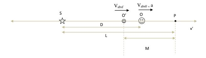
Suppose that, initially, at the instant of light emission, the observer was moving with initial absolute velocity  $V_{abs0}$ , at distance D from the source. Imagine that, just after emission of light, the observer starts accelerating to the right. The problem is to determine the time it takes light to catch up with the observer.
