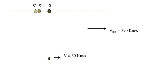
The sun will now appear to be at position S"( 20 arc seconds ahead of S'), due to Earth's *relative* motion. This is due to Bradley's aberration[37][38].
