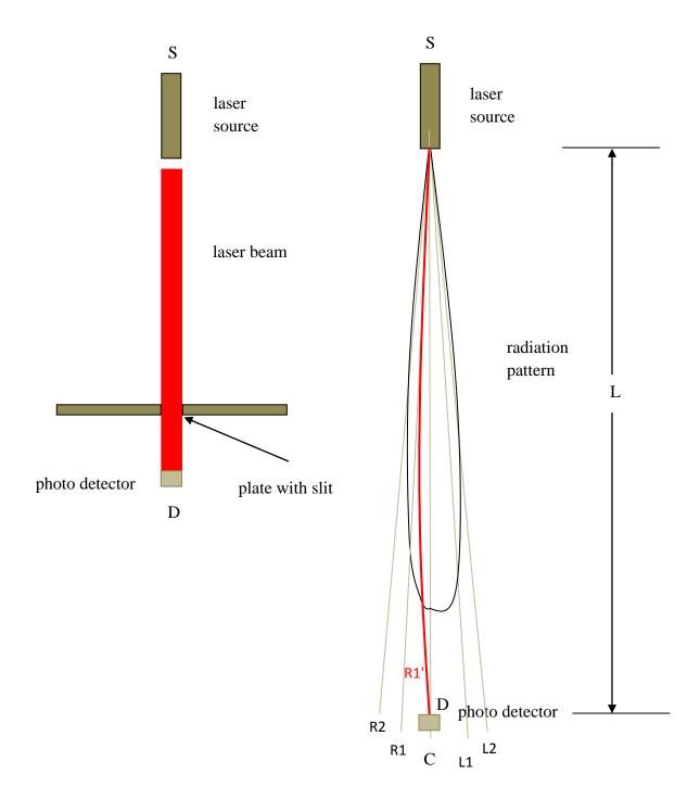
At first assume that there is no plate between the laser source and the photo detector. If the apparatus is at absolute rest and if the laser beam is aligned to the photo detector for maximum light intensity falling on the photo detector, the light ray going to the photo detector in this case will be ray C. Next assume that the apparatus is moving with absolute velocity to the
