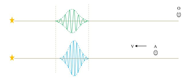
Consider two observers. Observer O is at rest relative to the light source and observer A is moving towards the light source. Observer A who is moving towards the light source should logically detect the light pulse earlier than the stationary observer O. However, observer A should observe a spatially compressed (smaller wavelength) form of the wave observed by stationary observer O, so that the phase velocity is always constant c relative to observe A.
