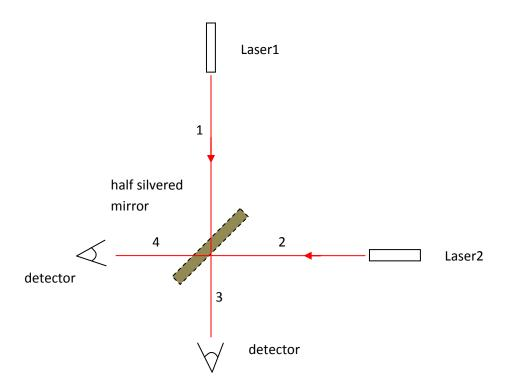
Consider the lasers to be ideal: their coherence time is infinite, and both have exactly the same frequencies and intensities, the arm lengths are exactly equal. The beam divergences are nearly zero.
