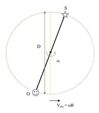
Our problem is to determine the path, the path length, the time delay and phase of a short pulse of light emitted by the source and detected by the observer.
