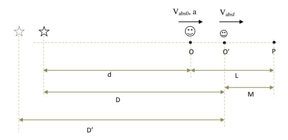
Let the accelerating observer be at point O at the instant of light emission (at t=0). Let us also assume that accelerating observer O will detect the light pulse at point P, which is a distance L from point O.
