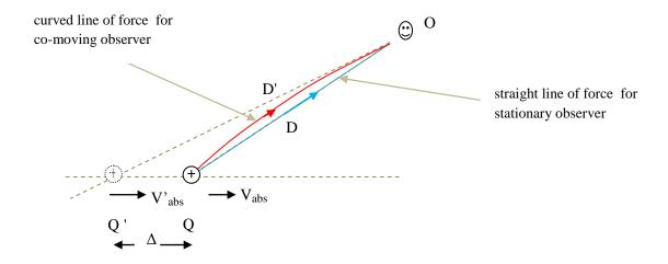
For the stationary observer, it is as if the electric field is rigidly carried by the moving charge, straight radial lines emanating from the charge.
