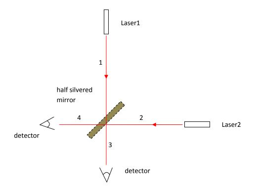
Consider the lasers to be ideal : their coherence time is infinite , and both have exactly the same frequencies and intensities, the arm lengths are exactly equal. The beam divergences are nearly zero.
