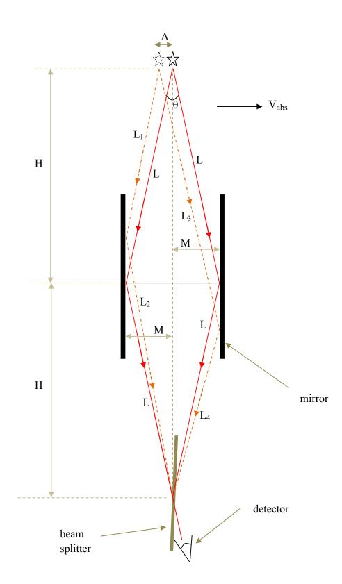
In the above experiment it is assumed that each photon has (nearly) equal probability of going to the right or to the left mirror. This is true for small angles  $\theta$ , but the experiment becomes less sensitive to absolute motion as angle  $\theta$  becomes small.
