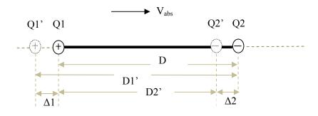
D is the actual, physical distance between real charges Q1 and Q2. D1' is the apparent distance of Q1 as seen by Q2. We can also say that D1' is the distance of apparent charge Q1' from real charge Q2. D2' is the apparent distance of Q2 as seen by Q1. We can also say that D2' is the distance of apparent charge Q2' from real charge Q1.
