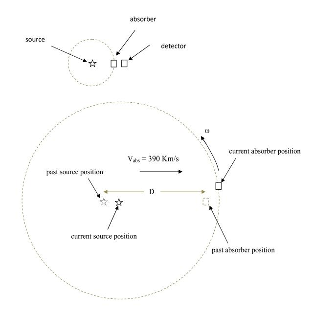
Why should we observe Doppler shift in the Mossbauer rotor experiment, as the source and detector are not in relative motion ? As stated in the last section, this is because the present observer ( at moment of detection) is moving relative to the past source (at moment of emission).
