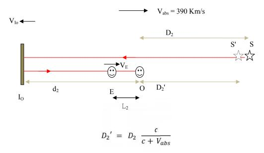
Suppose again that the source emits light at t = 0, while E is at the position shown ( the same initial position as the first case ). A co-moving observer O detects the light, after reflection from  $I_0$ , after a time delay of:
