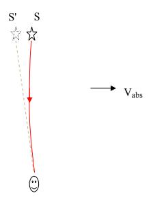
We see that the apparent change in position of the source is due to the curving of the light rays, as shown above. *The curve is determined by applying the Apparent Source Theory (AST) at every point*. Even though the source is physically, actually at position S relative to the observer, it appears to the observer that it is at position S' and this is due to the curving of the light ray which is a result of absolute velocity.
