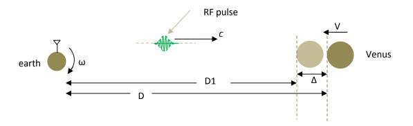
According to Special Relativity and ether theories, the center of the spherical wave fronts of the transmitted RF pulse remains at the point in space where the source was at the instant of emission. According to Apparent Source Theory, the center of the spherical wave fronts moves with the apparent source. As stated above, there is no significant difference between the real and the apparent positions of the source (the transmitter / antenna).
