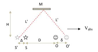
The time T elapsed for the light to travel from S', reflection at mirror, then arrive at O' is equal to the time taken for the observer to move from O to O'. The speed of light is c relative to the apparent source. We have to determine the speed of light c' in the dashed light ray, as seen in the absolute reference frame.
