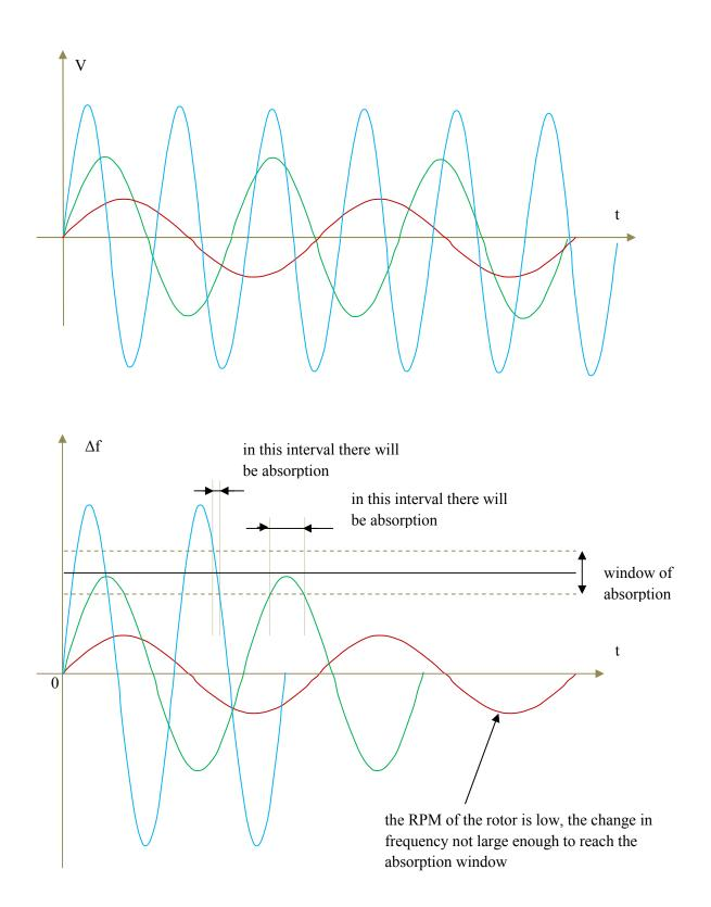
We assumed that there is no absorption at zero angular velocity, because the difference between the resonance frequencies of the source and the absorber is usually made slightly different.
