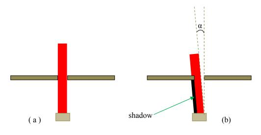
We can see that when the light is bent due to absolute motion, part of the light rays is blocked by the plate, creating a shadow and hence a decrease in intensity (quantity of light per unit area) of light falling on the photo detector. By measuring the voltage output of the photo detector, it is possible to observe variation of light intensity with variation in absolute velocity and with variation in orientation of line SD relative to the absolute velocity.
