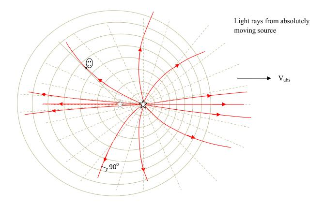
\* note that the above diagram is not drawn accurately. The light rays should always make  $90^{\circ}$  with the wave fronts. The bending light rays are only for a co-moving observer. For an observer at rest, light rays come as usual in straight lines from the point where they were emitted.
