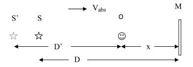
Time delay between emission and reception before reflection of light from mirror M, at point x, has been determined as follows (preceding section).
