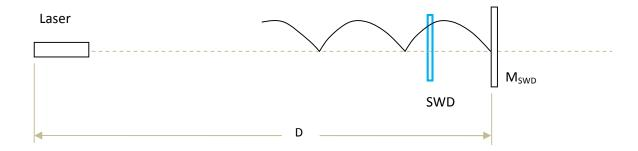
If we consider the whole optical system as a resonant cavity, then the distance D between the laser and the mirror becomes important. The standing wave will be maximum when D is an integral multiple of half wave lengths. If D is not equal to an integral multiple of half wave
