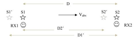
The operation of the clock is as follows: S1 emits a light pulse, then the detector RX2 detects the pulse, S2 transponds with another light pulse without delay, the detector RX1 detects the light pulse and S1 transponds without delay and so on. An electronic pulse counter can count the number of transmissions and hence a clock.
