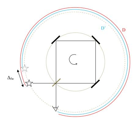
The red line represents 'direct' source detector distance D. The blue line is the apparent source detector distance D'.
