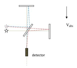
The blue and red dotted lines show the two light beams. The drawing is not meant to be accurate but only to illustrate the idea.
