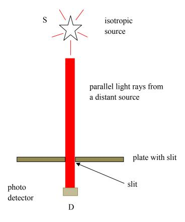
If the whole apparatus is at absolute rest, or if the line connecting the source and the photo detector (line SD) is oriented parallel to the absolute velocity vector, there will be no bending of the light ray.
