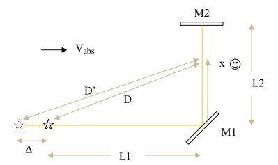
To analyze this problem, we first have to determine the apparent change in position ( $\Delta$ ) of the source as seen from point x, due to absolute motion.
