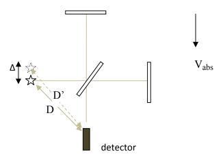
What is the effect of absolute velocity in this case? In the same way as above, we ask: what is the effect of actually, physically shifting the source from S to S'? In this case also there may be a very small fringe shift because the two beams will be misaligned and will have slightly different path lengths.
