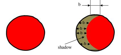
The left diagram shows a bright circular spot on the photo detector which will occur when there is no bending of the light ray. The right diagram shows what the spot of the light ray on the photo detector looks like, with a shadow due to bending of the light ray. Note that the size of the shadow has been exaggerated, which is actually only about 16.56% of the total area of the circle for an absolute velocity of 390 Km/s of the Earth.
