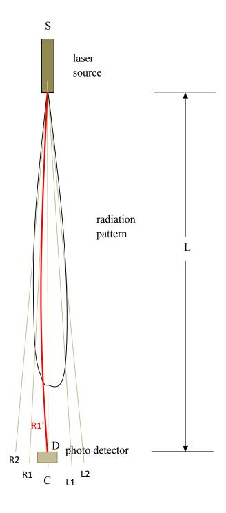
In this case, since the intensity of ray R1 ( R1' ) is less than intensity of ray C, then we detect a change in intensity at the detector due to absolute velocity.
