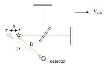
From the above diagram of the Michelson-Morley experiment, we see that the effect of absolute velocity is just to create an apparent change of the position of the light source relative to the detector, for absolute velocity  $V_{abs}$  directed to the right.
