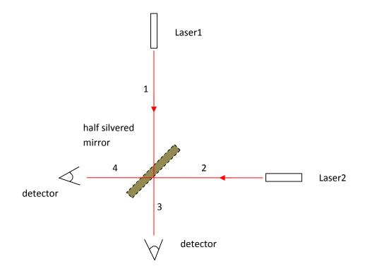
Consider the lasers to be ideal : their coherence time is infinite , and both have exactly the same frequencies and intensities, the arm lengths are exactly equal.
