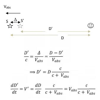
where V' is the velocity of the apparent source.
