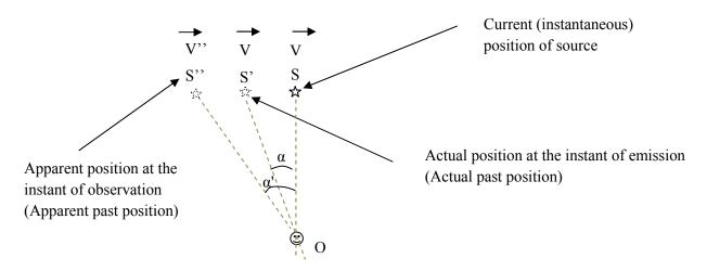
The source position now (at the moment of observation) is at S, moving with velocity V. But the source was at position S' at the moment of emission, moving with velocity V also, assuming uniform motion. The apparent position of the source at the moment of observation ( i.e. apparent
