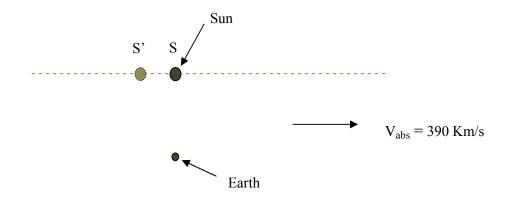
Assume that the Sun and the Earth are co-moving absolutely as shown above, with no relative motion between them. The amount of apparent change of the Sun's position is determined by the absolute velocity (390 km/s), the Earth-Sun distance and the speed of light. The light rays are coming from the direction of the apparent Sun (S').
