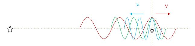
The green wave represents the wave for source and observer at rest relative to each other. The red and blue waves are for the cases of the observer moving away from the source and towards the source, respectively. Suppose that the observer is initially at rest relative to the source. He will observe the green wave. Now imagine that the observer accelerates instantaneously to velocity V towards the source. The wave observed by the observer will change instantaneously
