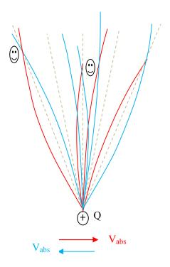
Since the lines of force are bending relative to the charge due to absolute motion, the lines of force will have *transverse* component. As the charge oscillates left and right, the observer in the reference frame of the charge observes that there is a time varying *transverse* component of the electric field, changing directions and magnitudes as the charge accelerates to the right and to the left. The time varying transverse component of the electric field causes electromagnetic
