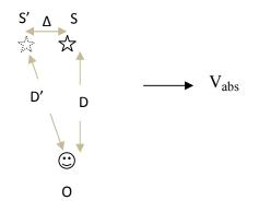
In this case also, the effect of absolute velocity is to create an apparent change in the *position* of the source relative to the observer.
