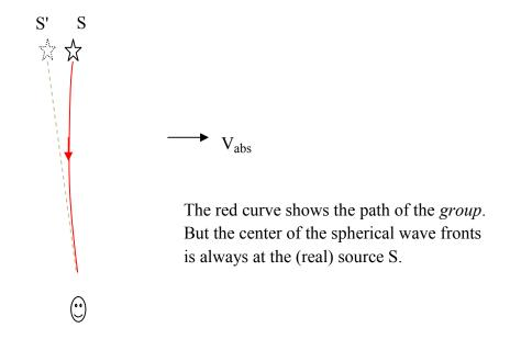
We see that the apparent change in position of the source is due to the curving of the light rays, as shown above. *The curve is determined by applying the Apparent Source Theory (AST) at every point*. Even though the source is physically, actually at position S relative to the observer, it appears to the observer that it is at position S' and this is due to the curving of the light ray which is a result of absolute motion.
