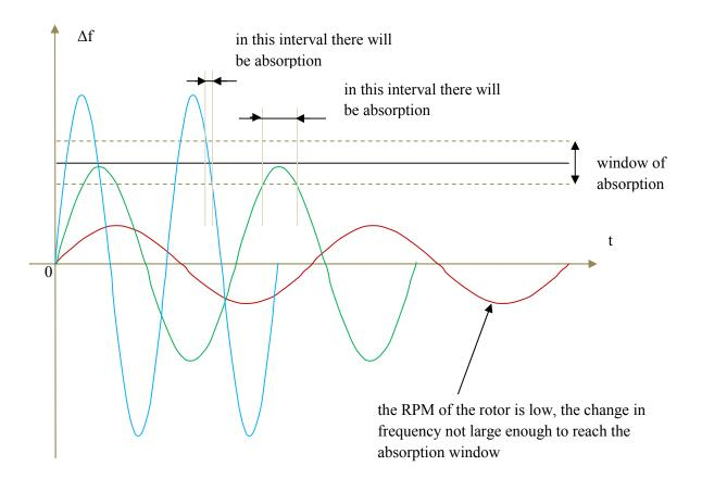
We assumed that there is no absorption at zero angular velocity, due to difference between the resonance frequencies of the source and the absorber, i.e. source is different from absorber.
