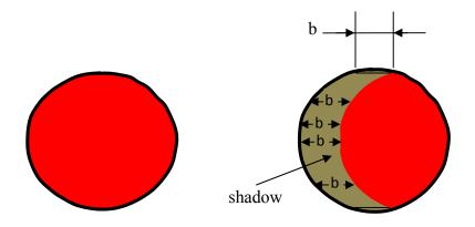
The left diagram shows a bright circular spot on the photo detector which will occur when there is no bending of the light ray. The right diagram shows what the spot of the light ray on the photo detector looks like, with a shadow due to bending of the light ray. Note that the size of the shadow has been exaggerated, which is actually only about 16.56% of the total area of the circle for an absolute velocity of 390 Km/s of the Earth.
