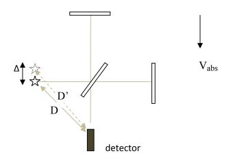
What is the effect of absolute velocity in this case? In the same way as above, we ask: what is the effect of actually, physically shifting the source from S to S', assuming Galilean space and/or emission theory? In this case there will be a small fringe shift because the two beams will be misaligned and will have different path lengths.
