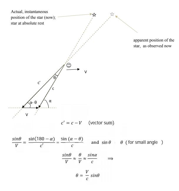
This is the kind of aberration known as Bradley aberration. In this case, aberration is due to the difference between the actual (instantaneous) and apparent position of the star, caused by the motion of the observer. In this case star light aberration is an apparent change of <u>current</u> (instantaneous) position of the star. This is only an illusion, like a man running in rain with rain drops appearing to fall in slant path.
