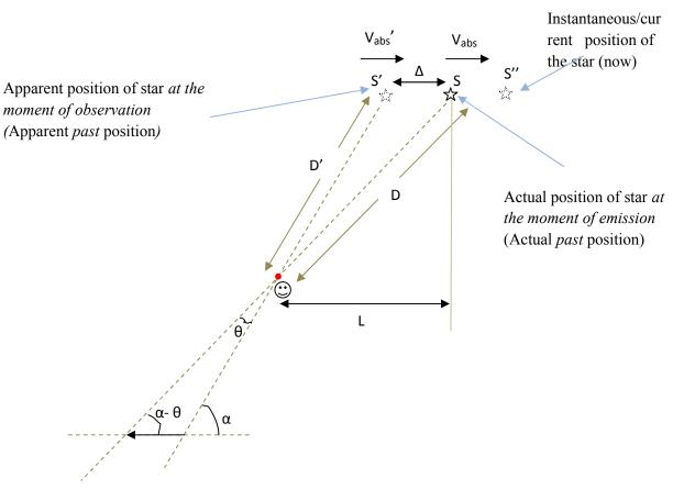
From the above two equations, D' and  $\Delta$  can be determined (it is a lengthy formula), and then the angle of aberration  $\theta$  can be determined. Note that angle  $\theta$  is due to a difference in the actual past position of the star and its apparent past position, as seen at the time of observation. Unlike conventional explanations, the current (instantaneous) position of the star has no role in the explanation of stellar aberration.
