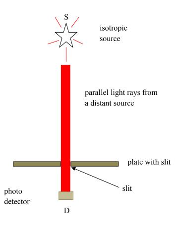
If the whole apparatus is at absolute rest, or if the line connecting the source and the photo detector (line SD) is oriented parallel to the absolute velocity vector, there will be no bending of the light ray.
