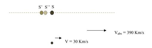
The sun will now appear to be at position S"(20 arcseconds ahead of S'), due to earth's *relative* motion. However, this does not mean that the light rays are coming from the direction of S''; it is only an illusion. The light rays still come from the direction S'. It appears to a person running in
