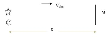
The light source emits a short light pulse towards the mirror. The reflected light is detected by the detector, which triggers the light source to emit another light pulse and so on. A counter counts the number of round trips.
