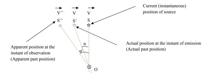
The source position now (at the moment of observation) is at S, moving with velocity V. But the source was at position S' at the moment of emission, moving with velocity V also, assuming
