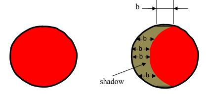
The left diagram shows a bright circular spot on the photo detector which will occur when there is no bending of the light ray. The right diagram shows what the spot of the light ray on the
