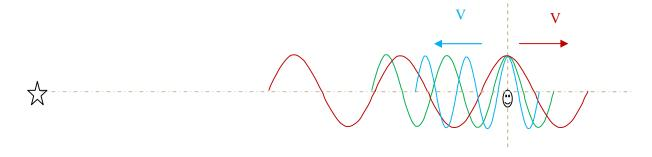
The green wave represents the wave for source and observer at rest relative to each other. The red and blue waves are for the cases of the observer moving away from the source and towards the source, respectively. Suppose that the observer is initially at rest relative to the source. He will observe the green wave. Now imagine that the observer accelerates instantaneously to
