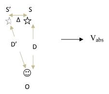
In this case also, the effect of absolute velocity is to create an apparent change in the *position* of the source relative to the observer.
