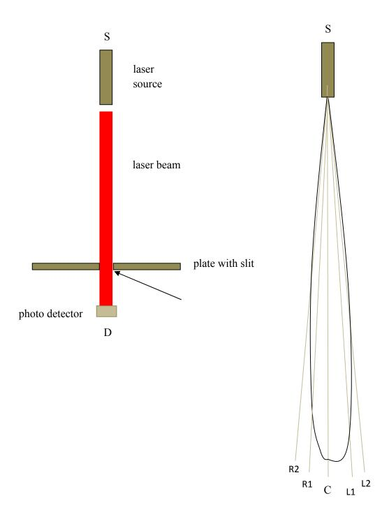
At first assume that there is no plate between the laser source and the photo detector. If the apparatus is at absolute rest and if the laser beam is aligned to the photo detector for maximum light intensity falling on the photo detector. The light ray going to the photo detector in this case will be ray C. Next assume that the apparatus is moving with absolute velocity to the right, without changing the alignment of the laser beam. In this case it will be light ray R1 that
