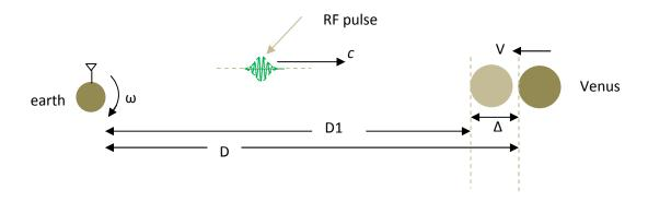
According to Special Relativity and ether theories, the center of the spherical wave fronts of the transmitted RF pulse remains at the point in space where the source was at the instant of emission. According to Apparent Source Theory, the center of the spherical wave fronts moves with the apparent source. As stated above, there is no significant difference between the real and the apparent positions of the source (the transmitter / antenna).
