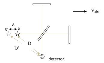
From the above diagram, we see that the effect of absolute velocity is just to create an apparent shift of the position of the light source relative to the detector, for absolute velocity  $V_{abs}$  directed to the right.
