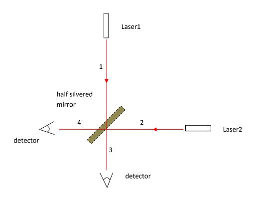
Consider the lasers to be ideal: their coherence time is infinite, and both have exactly the same frequencies and intensities, the arm lengths are exactly equal.
