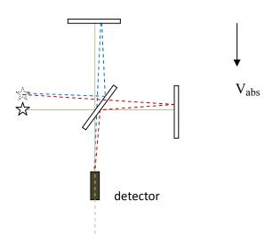
The blue and red dotted lines show the two beams. The drawing is not drawn to be accurate but only to illustrate the idea.
