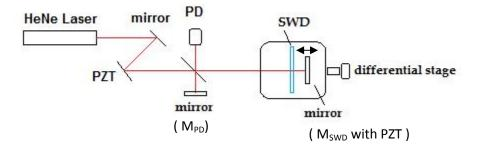
Doug Marett reported that he detected phase shift of the SWD voltage as the stage is moved, with the mirror  $M_{SWD}$  and the SWD detector co-moving with the stage. The  $M_{SWD}$  is also actuated with a triangle wave. He used the above arrangement.
