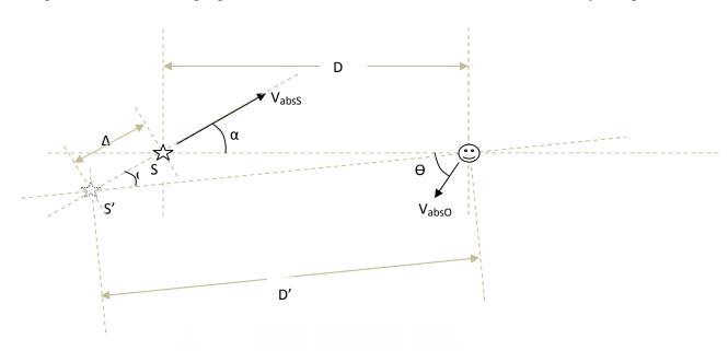
$$V = V_{absS}cos\alpha + V_{absO}cos\theta$$
