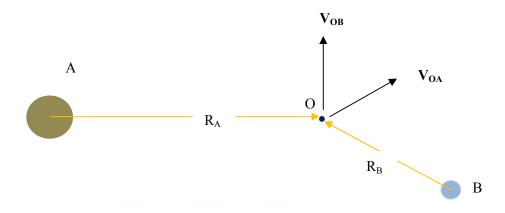
$$V_{abs} = \frac{M_A}{M_T} V_{OA} + \frac{M_B}{M_T} V_{OB}$$
