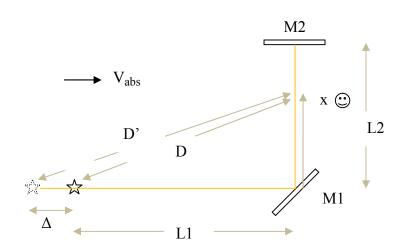
To analyze this problem, we first have to determine the change  $(\Delta)$  in apparent position of the source as seen from point x, due to absolute motion.
