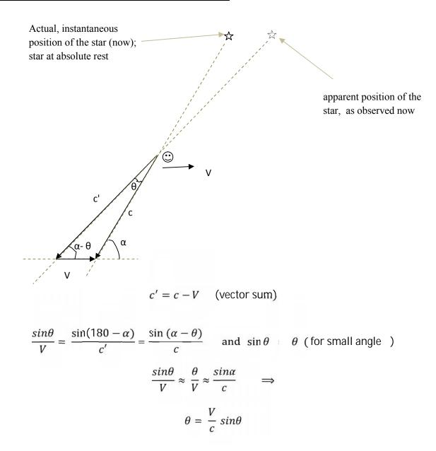
This is the kind of aberration known as Bradley aberration. In this case, aberration is due to the difference between the actual (instantaneous) and apparent position of the star, caused by the motion of the observer. In this case star light aberration is an apparent change of *current* (instantaneous) position of the star. This is only an illusion, like a man running in rain with rain drops appearing to fall in slant path.
