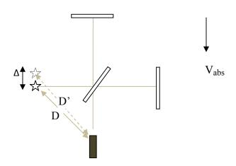
What is the effect of absolute velocity in detector the same way as above, we ask: what is the effect of actually, physically shifting the source from S to S', assuming Galilean space and/or emission theory? In this case there will be a small fringe shift because the two beams will be misaligned and will have different path lengths.
