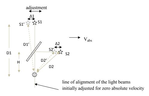
With zero absolute velocity, the two light beams arriving at the detector are adjusted to be aligned. Then, with non zero absolute velocity, the two beams will be misaligned and a fringe shift will occur. The position of the source S1 may be adjusted (towards the right) until the two light beams are aligned again. The amount of adjustment of position of S1 required to align the two beams again can be used to determine the absolute velocity.
