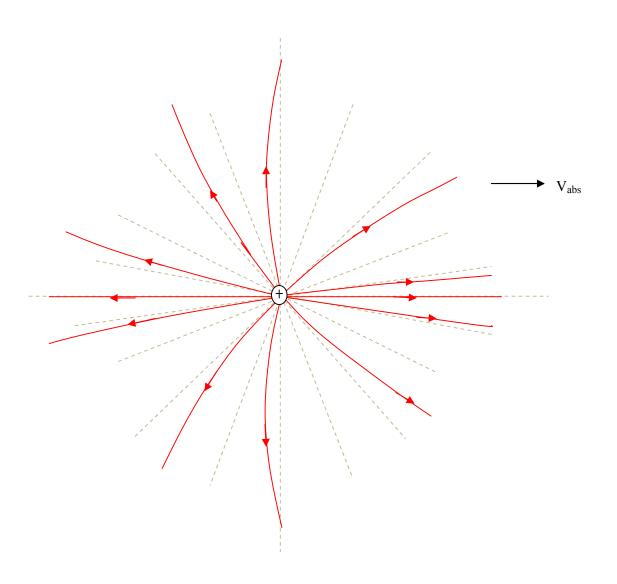
From the above figure, we see that bending of the light rays is maximum in lateral directions, at or near the ninety degrees (orthogonal) directions. In the forward and backward directions ( $0^0$  and  $180^0$ ), there is no bending of the light rays. In directions close to these directions, for example  $2^0$  or  $178^0$ , there is a very slight bending only.
