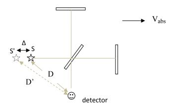
From the above diagram, we see that the effect of absolute velocity is just to create an apparent shift of the position of the light source relative to the detector, for absolute velocity  $V_{abs}$  directed to the right.
