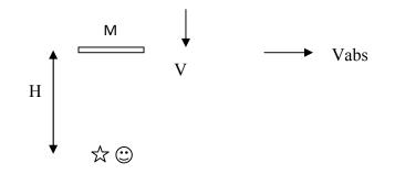
If the mirror is not moving, the round trip time of a light pulse emitted by the source will be:  $T_d = 2H/c$
