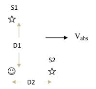
S1, S2 and observer O are co-moving absolutely to the right with absolute velocity  $V_{abs}$ . If  $V_{abs}$  is zero the two time delays will be equal.
