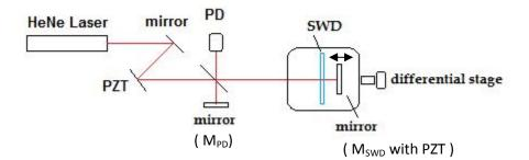
Doug Marett reported that he detected phase shift of the SWD voltage as the stage is moved, with the mirror  $M_{SWD}$  and the SWD detector co-moving with the stage. The  $M_{SWD}$  is also actuated with a triangle wave. He used the above arrangement.
