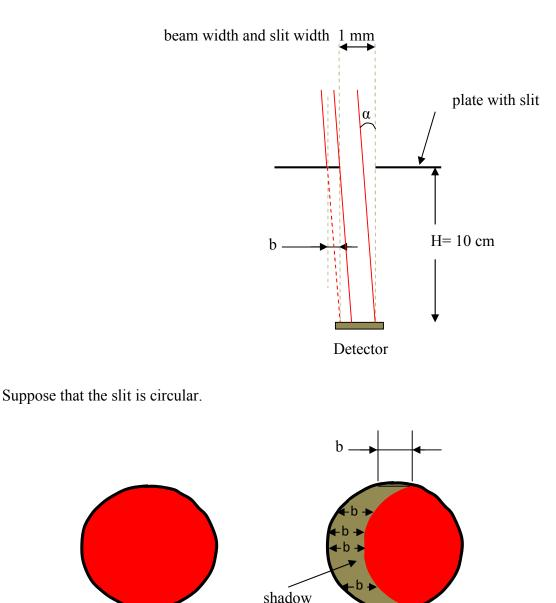
The left diagram shows a bright circular spot on the photo diode which will occur when there is no bending of the light ray. The right diagram shows what the spot of the light ray on the photo diode looks like, with a shadow due to bending of the light ray. Note that the size of the shadow has been exaggerated, which is actually only about 16.56% of the total area of the circle for an absolute velocity of 390 Km/s of the Earth.
