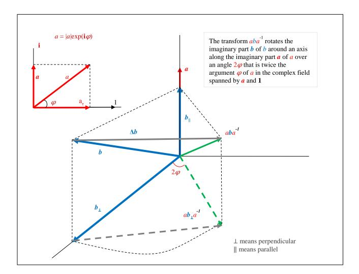
This means that if  $\varphi = \pi/4$ , then the rotation c = a b/a shifts  $b_{\perp}$  to another dimension. This fact puts quaternions that feature the same size of the real part as the size of the imaginary part is in a special category. They can switch states of tri-state systems.
