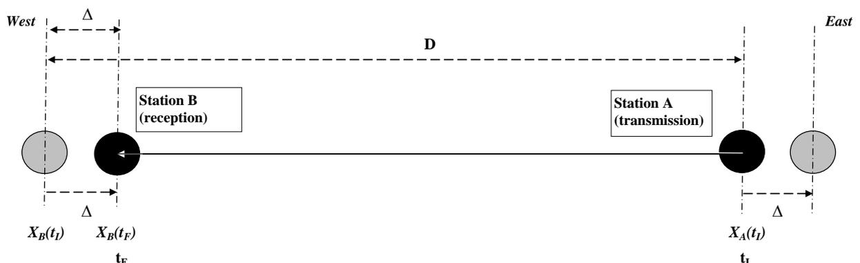
Fig.2. One-way light speed determination – westward transmission
