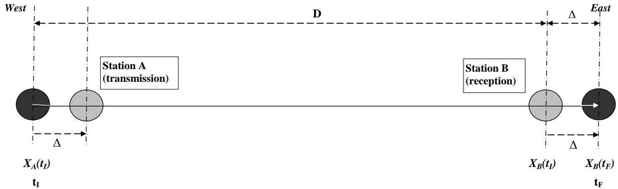
Fig.1. One-way light speed determination – eastward transmission
