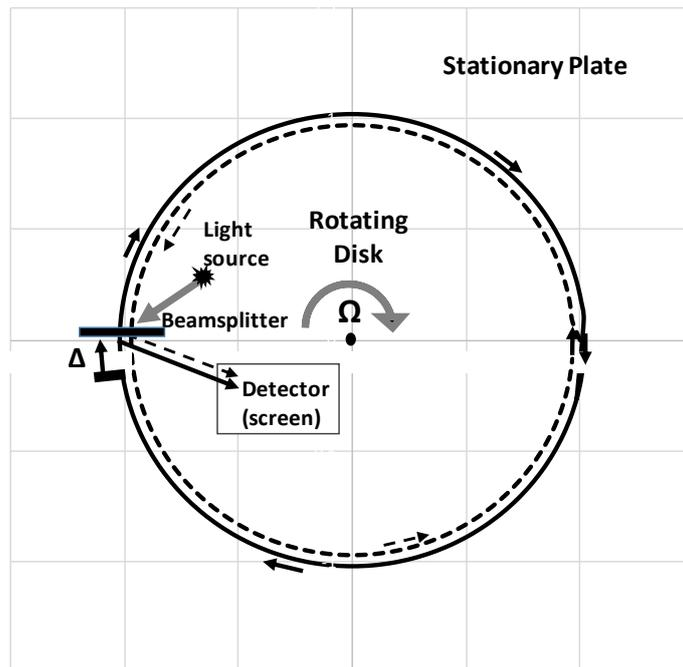
Fig.4 Schematic representation of a fiber optic interferometer
