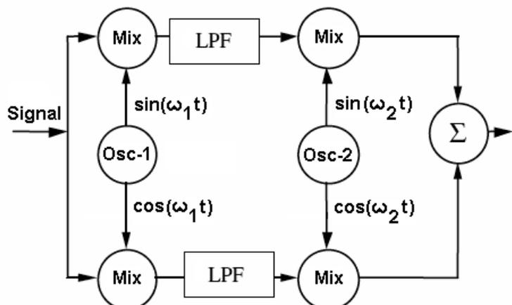
spectral frequency may be shifted to any predetermined value. Here, the signal frequency will be shifted so that it exactly matches a frequency bin of the downstream FFT. In radio-frequency technology, the corresponding principle is a superheterodyne receiver, where the signal frequency is shifted to a better processable intermediate frequency without changing the message content.
