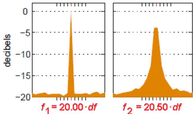
In the left picture, the frequency of a noisy signal is exactly 20 times the fundamental frequency  $df$  of the FFT analysis. At the junction of successive data sequences, there is no phase discontinuity. The peak is exactly one bin wide without spectral leakage to neighboring frequencies. A dream result! A Dirac delta function and not a wide bell curve with blurred peak.
