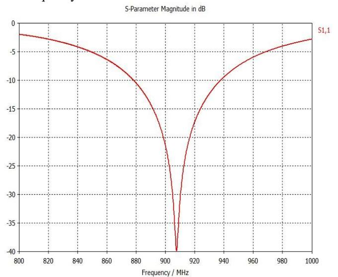
Fig. 2 Displays return loss contrasted with frequency
