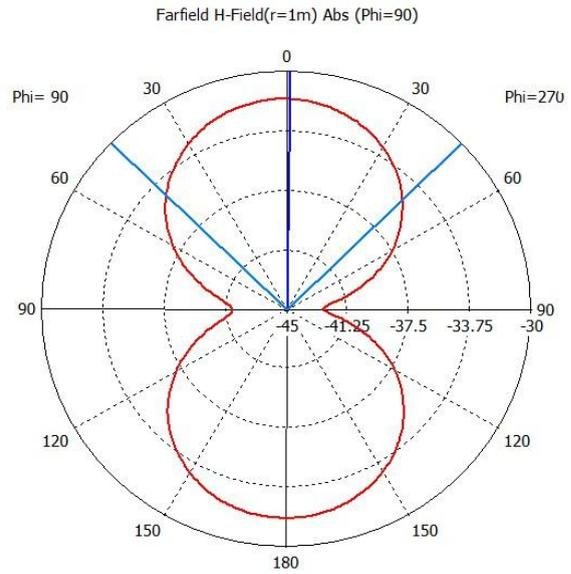
Fig. 4(b). H-field of proposed antenna
