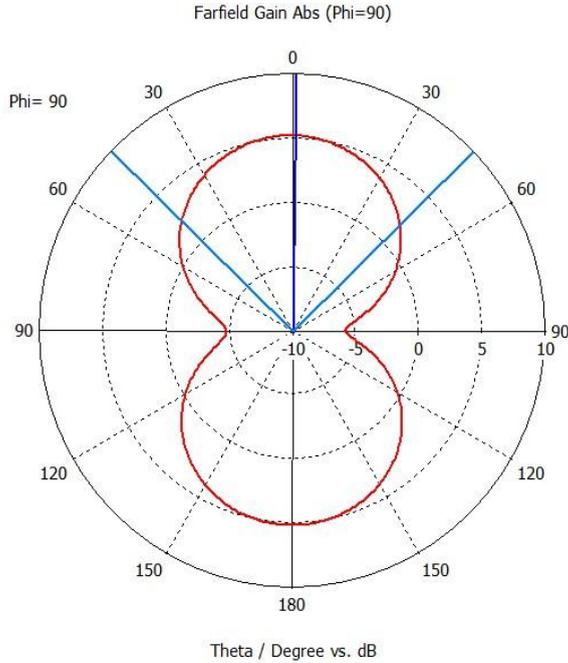
Fig. 3 Gain of proposed Antenna
