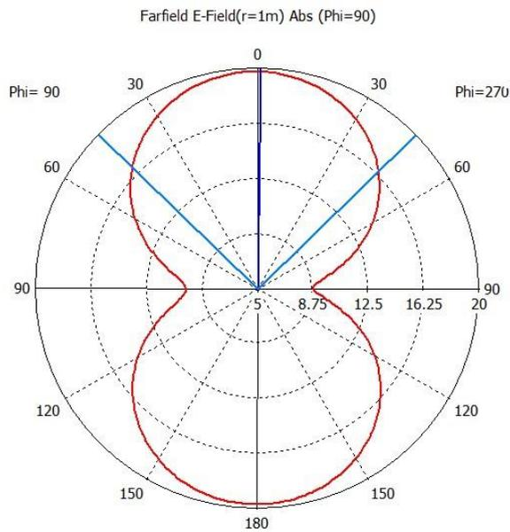
Fig 4(a). E-Field of Proposed Antenna
