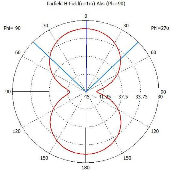
Fig. 4(b). H-field of proposed antenna
