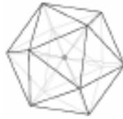
The 2-shell 55-atom Pd/Ni cluster (1.13 nm) is the next level of icosahedral structure. It contains two 13-atom icosahedra that share a central vertex:
