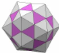
The 3-shell 147-atom Pd/Ni cluster (1.56 nm) is the next larger icosahedral structure. It contains 12 exterior 13-atom icosahedra plus 1 central 13-atom icosahedron whose 12 outer vertices are shared, each with one vertex of the 12 exterior icosahedra:
