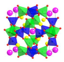
It shows that of the 24 vertices of the sodalite cage, 12 are Aluminum and 12 are Silicon so each Zeolite Cavity has 10 x 12 = 120 Aluminum atoms.
