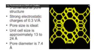
A corresponding enlargement of pore size is to about 1.5 nm which would permit a 3-shell 147-atom Palladium cluster to enter the Zeolite Cavity.
