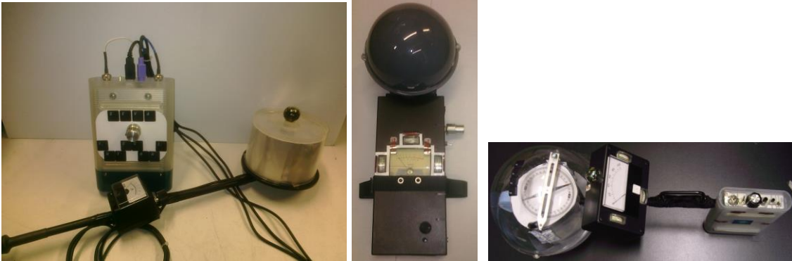
Fig.2. Some of the instruments of the later versions of SEVA. These instruments are wide-band ones, from ELF up to 600kHz.
