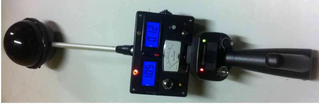
Fig.4. SEVA-Integral-M1 –the latest model of the family, up to 250 MHz. This is a very first model, where stationary and non-stationary rotations are separated, having 2 separate readouts (blue DVM) and the channels of recording. The instrument also has an ELF unit.
