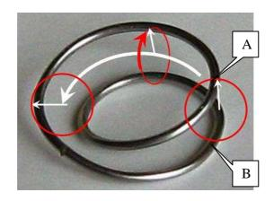
The helix is made of two pieces, the first piece from A to B rotates 180 degrees and the second, from B to A, again 180 degrees.
