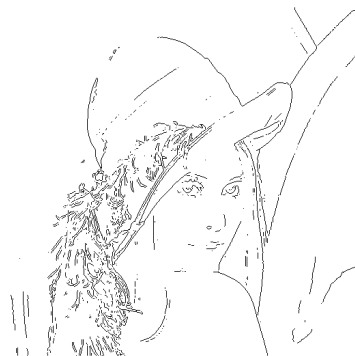
Figure 7. Sobel's edge detector on Lena's gray image.
