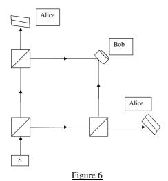
Figure 6 shows an arrangement with three beamsplitters and two measuring gates (though only one gate need be used). It is not to difficult to imagine ways that the paths of Alice and Bob can be brought out from the closed arrangement and sent in opposite directions by mirrors.
