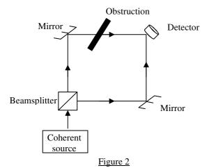
A re-arrangement of the interferometer can then effect the communication of classical digital data over a quantum channel[5] by interfering one output port of the interferometer with another coherent source.
