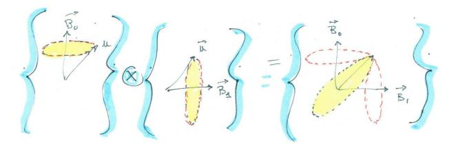
The diagram on the left shows  $\vec{L}$  precessing with Larmor frequency  $\omega_0$  in a uniform magnetic field,  $\vec{B}_0$ . The middle diagram shows a second (orthogonal) magnetic field designed to rotate with angular frequency  $\omega$  about fixed field  $\vec{B}_0$ .
