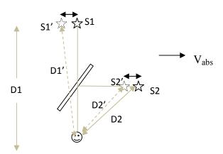
With zero absolute velocity, the two light beams arriving at the detector are aligned and have equal path lengths. However, with non zero absolute velocity, the two beams will be misaligned and there will be a difference in the path lengths of the two beams , hence a fringe shift will be expected.
