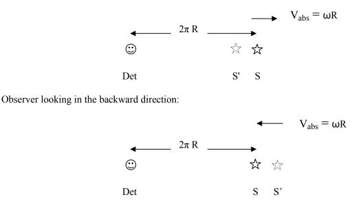
If the device is at absolute rest, i.e. not in rotation (and not in absolute translational motion), the observer sees the light source to be at its real position S.
