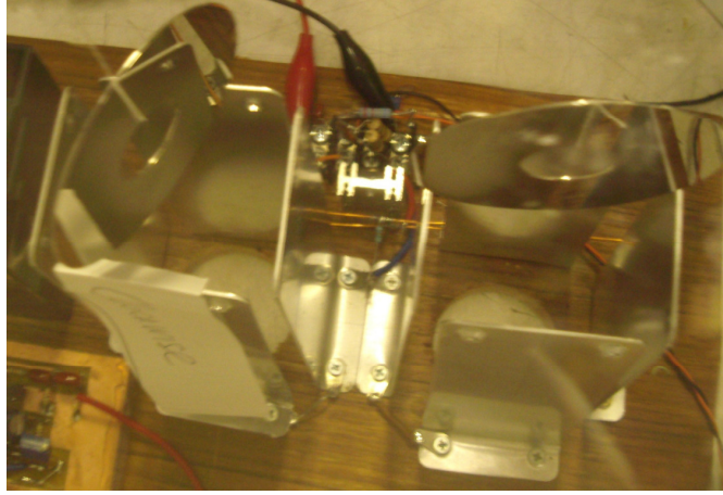
Fig.6. Two quadrupole spinners, generating opposite modulated spinning electric fields 400V/m @3MHz, according to Fig.1, having the disks placed in the originated FG. During the experiment, the disks turned for as much as 10 degrees.
