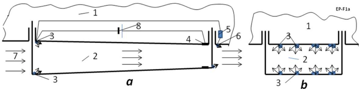
**Fig.1.** Electron ramjet engine (ABEP). *a* – side view, *b* – forward view. *Notations:* 1 – aircraft body, 2 – propulsion body, 3 – injector of charges (forward electrode), 4 – back electrode, 5 - separator (compensator) of charges; 6 – back injector of charges (opposed the forward injector 3), 7 – air flow. 8 – issue of high voltage (example, the electrostatic generator).
