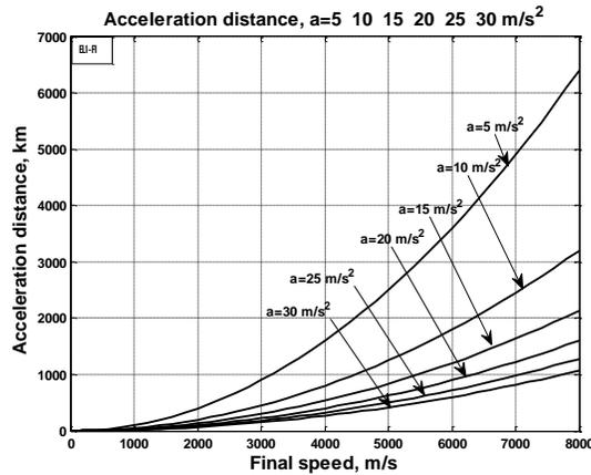
**Fig. 7.** Acceleration distance of hypersonic aircraft via final speed of ABEP for different acceleration  $\text{m/s}^2$ .
