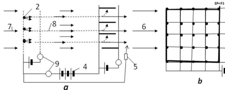
**Fig.3.** The electrical circuit of one version ABEP engine. Notations: *a* is side view, *b* is forward view; 2 – injector; 4 – electric issue, for example, the electrostatic generator, 5 – Compensator; 6 - exit flow, 7 – air flow, 8 – trajectory of the charges, 9 – regulator.
