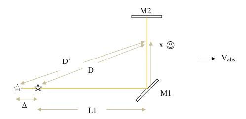
To analyze this problem, we first have to determine the change ( $\Delta$ ) in apparent position of the source due to absolute motion.
