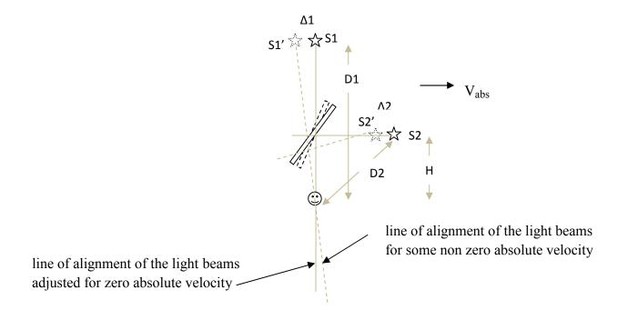
Let the two light sources be at distances D1 and D2 from the detector. Note that D1 and D2 are the *direct* distances between the detector and the sources and not between the mirror and the sources.
