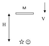
If the mirror is not moving, the round trip time of a light pulse emitted by the source will be:  $T_d = 2H/c$
