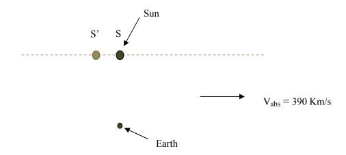
Assume that the Sun and the Earth move absolutely as shown above, with no relative motion between them. The amount of apparent change of the Sun's position is determined by the absolute velocity (390 km/s), the Earth-Sun distance and the speed of light. The light rays are coming from the direction of the apparent Sun (S').
