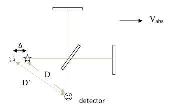
From the above diagram, we see that the effect of absolute velocity is just to create an apparent shift of the position of the light source, for absolute velocity Vabs directed to the right. Therefore, the apparent shift of the source is common both to the forward and lateral beams and hence the path lengths of both beams are affected in the same way and hence no fringe shift will occur.
