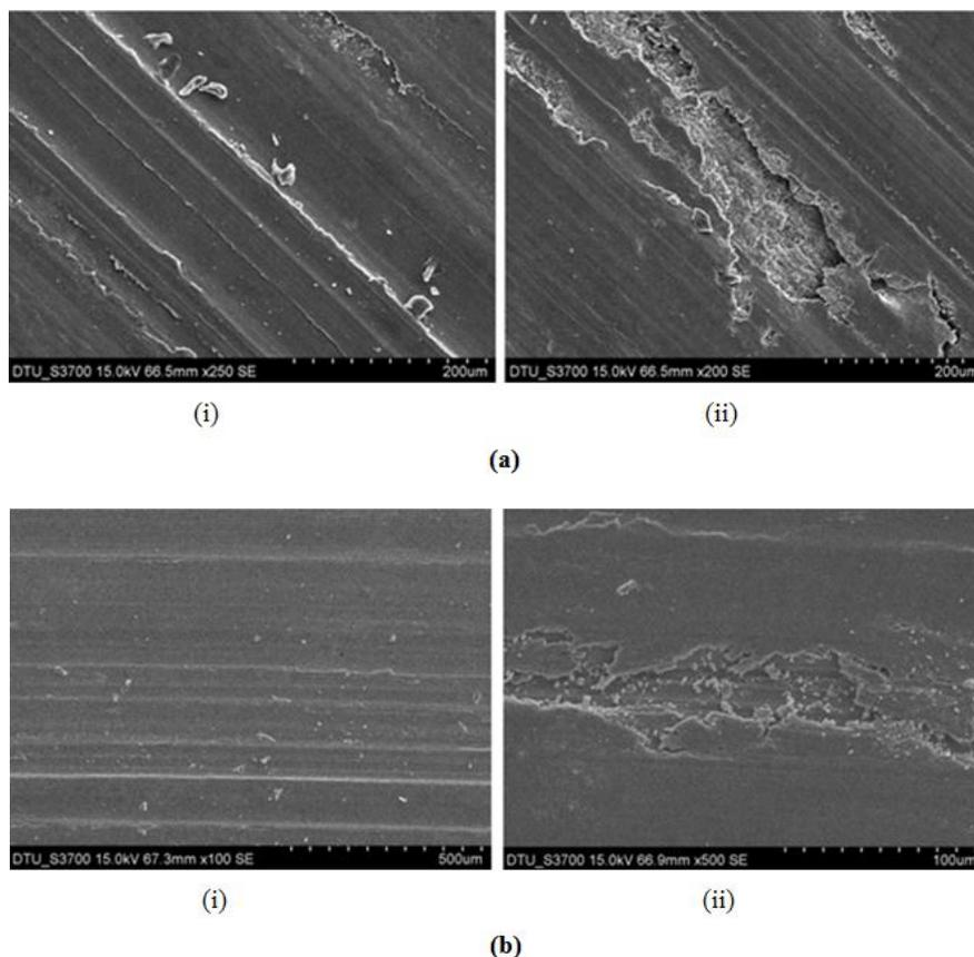
Fig. 9 Scanning electron micrographs of worn track: (a) 5083Al and (b) FSPed alloy specimens
