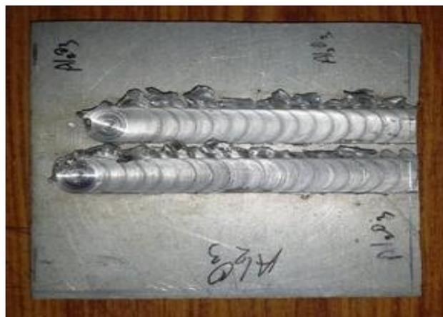
Fig. 3 Image showing tunneling effect in friction stir processed 5083Al Plate
