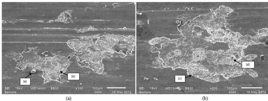
Fig. 10 SEM of worn track of 5083 Al sample
