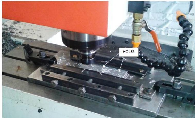
Fig. 2 Drilling holes on the top surface of base plate
