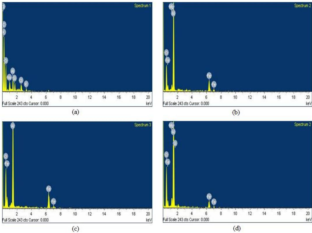
Fig. 11 EDS of wear debris of 5083Al at locations marked in Fig. 10
