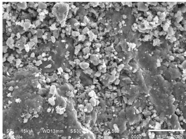
Fig. 12 SEM of worn track of FSPed sample
