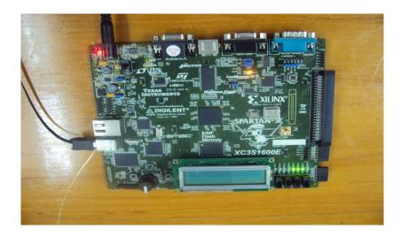
Fig. 5. Spartan-3E FPGA development kit
