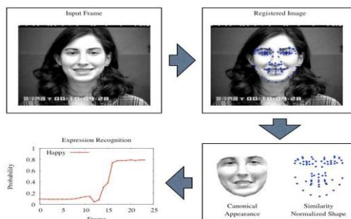
Figure 8: Automatic Facial Expression Recognition System. Similarity normalized shape and canonical appearance are estimated for each video frame. Parameters are then inputted to SVMs to recognize emotion expression on a frame-by-frame basis.
