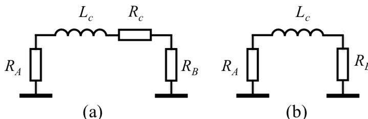
**Figure 2.** Lumped impedance-components-based model of a cable [2] at low frequencies for analyzing voltage drop along the cable and phase shift in the quasi static limit. Part (a) represents a cable with loss (cable inductance and resistance are designated  $L_c$  and  $R_c$ , respectively), and part (b) represents a lossless cable.
