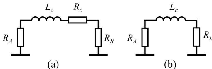
**Figure 2.** Lumped impedance-components-based model of a cable [2] at low frequencies for analyzing voltage drop along the cable and phase shift in the quasi static limit. Part (a) represents a cable with loss (cable inductance and resistance are designated  $L_c$  and  $R_c$ , respectively), and part (b) represents a lossless cable.
