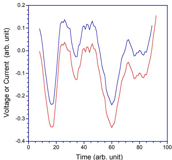
**Figure 3.** Computer generated example to illustrate how can a DC shift distinguish two strongly correlated noises by using a very short sample. If the DC shift is greater than the stochastic difference between the time functions then a *single-time measurement is enough to distinguish the two noises* and the bit situations in KLJN.
