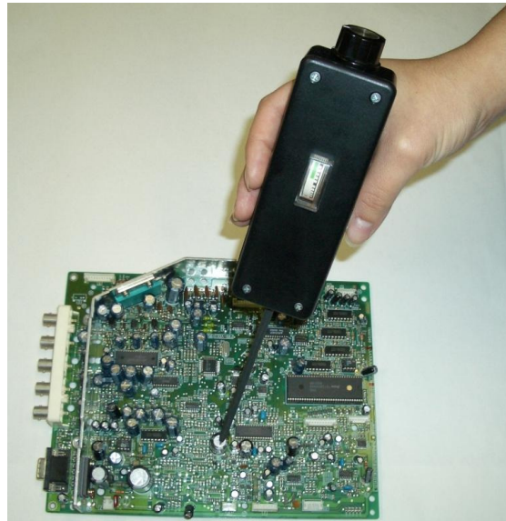
Fig.7. Measuring quality of capacitors with C-Miracle instrument. The instrument measures a quality Q=1/\text{tg}\delta
