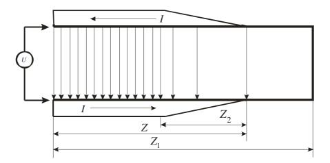
Fig. 1 . Propagation of the current wave and voltage in the long line.
