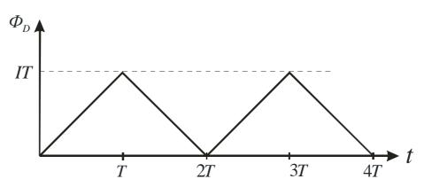
Fig. 4. Dependence of the electric flux on the time for the shortened transmission line.
