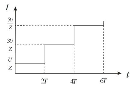
Fig. 2. Dependences of input current on the time for the shortened transmission line.
