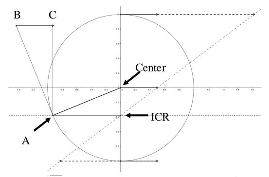
Figure 4. The line  $\overline{AB}$  is perpendicular to the line connecting the center of the circle to a point on the curcumference, point A. Line  $\overline{AC}$  is perpendicular to the line connecting the instant cneter of rotation to point A. Line  $\overline{BC}$  represents the lineal velocity vector,  $\overline{AB}$  is the tangential velocity vector, and  $\overline{AC}$  is the centripetal velocity vector. This example represents a spinning object moving at 0.5c to the right.
