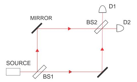
FIG. 1: A Mach-Zehnder interferometer: In standard quantum mechanics, the probability wave of the photon divides at beamsplitter BS1. Self interference then occurs as the partial probability waves recombine at BS2. In the local realistic explanation here, the scattering of the photon into one or other arm at BS1 induces by reaction secondary radiation precisely anticorrelated with the change in the photon and capable of interference with the photon at BS2.
