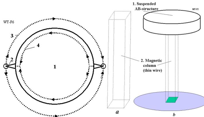
*Left.* Trans-continental wireless electric power transmission and Electricity storage ([30], [1], Ch.6). Using the ionosphere as a conducting medium for transferring a huge electric energy between continents and as a large capacity storage ‘battery’ for electric energy. *Notations:* 1 - Earth, 2 - space towers about 100 km of height, 3 - conducting E layer of Earth's ionosphere, 4 - back connection through Earth.
