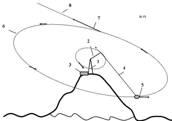
Centrifugal (Sling rotary) space launcher ([2], Ch.10). Launcher locates on mountain. Notations: 1 – tower, 2 – lever or disk, 3 – engine, 4 – sling, 5 – space apparatus (s.a.), 6 – circular launch trajectory, 7 – point of disconnection, 8 – direction of launch,
