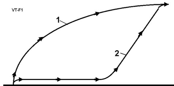
Vertical Takeoff and Landing aircraft trajectories: 1 – The original trajectory; 2 – The optimized trajectory (result of my research).
