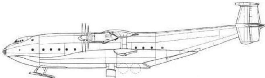
The project of the amphibian transport hydrofoil craft AN-22 developed by the experimental design bureau of Oleg Antonov.
