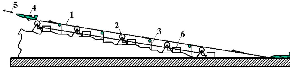
A fixed slope small launcher for projectiles. ([3], Ch.2). . Notation: 1 – cable contains 3 parts: main part, outlet part, and directive part; 2 – power drive station; 3 – cable support columns; 4 – winged space apparatus (space ship, missile, probe, projectile and so on); 5 – trajectory of space apparatus; 6 – engine.
