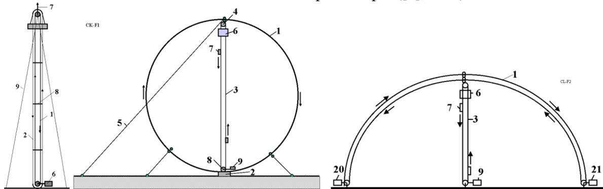
*Left:* Circle launcher and space station keeper. Notations are: 1 – cable circle, 2 – main engine, 3 – transport system, 4 – top roller, 5 – additional cable, 6 – the load (space station), 7 – mobile cabin, 8 – lower roller, 9 – engine of the transport system.
