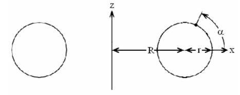
Define the inner, *I*, and outer/external/equatorial, *O*, radii of a torus I = R - r, O = R + r. Define following "action"
