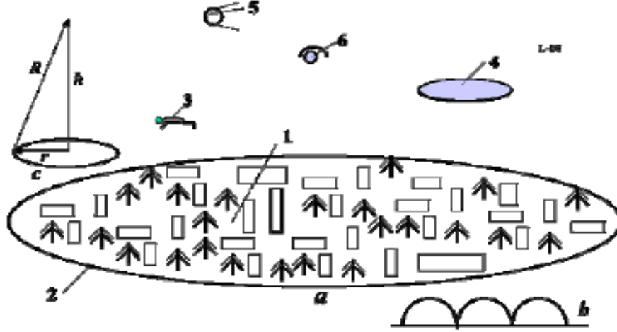
Figure 8. Artificial magnetic field. (a) City having the superconductivity electric ring. (b) Variation intensity of the magnetic field. Notation: 1 - city, 2 - superconductivity electric ring, 3 - flight man, 4 - levitator in the form of a flight plate (UFO), 5 - Earth's satellite, 6 - levitative illumination lamp. R = \rho in Eq. (16).
