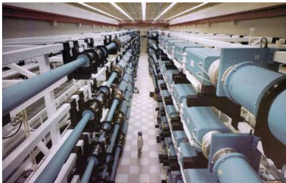
Figure 1. Laser installation for NOVA inertial thermonuclear reactor. Note the size of the man in comparison to the gigantic size of the class of laser installation needed for a reactor. Cost is some billions of dollars.
