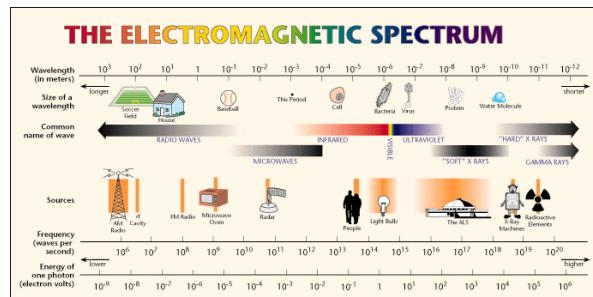
Figure 2. The Electromagnetic Spectrum
