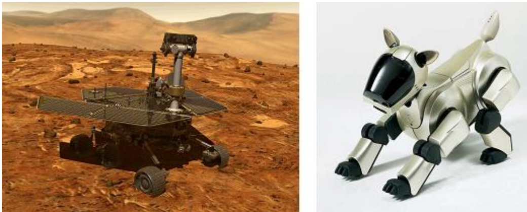
Fig : 23 Robotic systems; NASA (National Aeronautics and Space Administration) Mars Rover Spirit (Left) and Sony AIBO Entertainment Robot (Right). Both robots make use of feedback between sensors, actuators, and computation to function in unknown environments. These are also examples of Dynamical Systems.
