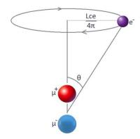
In this "Cone" model of an electron, the orbital angular momentum L equals to spin  $s=\frac{h}{4\pi}$ , and the orbital magnetic dipole momentum equals to  $\frac{\mu_B}{2}$ . The dipole momentum of the magnetic dipole also equals to  $\frac{\mu_B}{2}$  (3.2.13). The total magnetic momentum then equals to  $\mu_B$  – the Bohr magneton.
