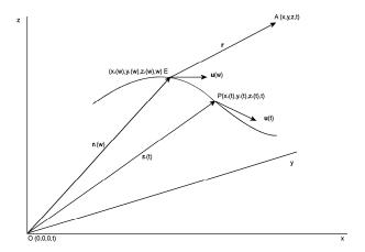
**Figure 2.2.1** Material point particle in arbitrary motion. As the material particle moves from point  $E(x_p(w), y_p(w), z_p(w), w)$  to point  $P(x_p(t), y_p(t), z_p(t), t)$ , a generalized photon moves from point  $E(x_p(w), y_p(w), z_p(w), w)$  to point A(x, y, z, t).
