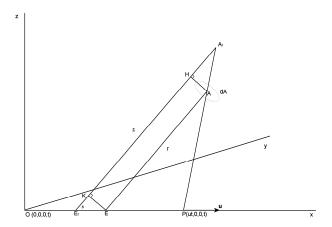
**Figure 3.5.2** Figure 3.5.1 as modulated in the inertial reference frame S(0, x, y, z, t), in which the material particle moves with constant speed. The points P, A and  $A_1$ remain collinear, as results from the Lorentz-Einstein transformations.
