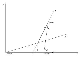
**Figure 3.2.1** Material point particle moving with constant speed along the x axis of the inertial reference frame S(0, x, y, z, t). As the material particle moves from point
