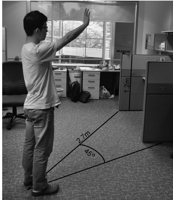
Figure 1: Experimental Setup: the user is facing the camera at angle of 45^\circ to the right of the sensor. Every arm movement is recorded at fixed 2.7 m distance from the camera; where the camera is placed at height of 1.2 m above the floor.
