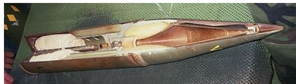
Figure 2 (left): Sections 1: Aerodynamic cover; 2: Empty cavity; 3: Conical liner; 4: Detonator; 5: Explosive; 6: Piezo-electric trigger Figure 3 (Top-right). Work of shaped charge.
