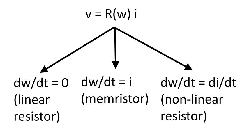
Are mem-capacitor and mem-inductor the 5<sup>th</sup> and 6<sup>th</sup> "fundamental" circuit elements?
