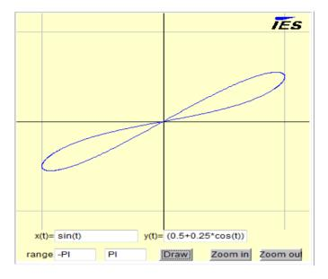
In this example the voltage amplitude is reduced to half of that in Example 1. The hysteresis curve begins to degenerate as the amplitude is reduced similarly to the behavior of the theoretical memristor.
