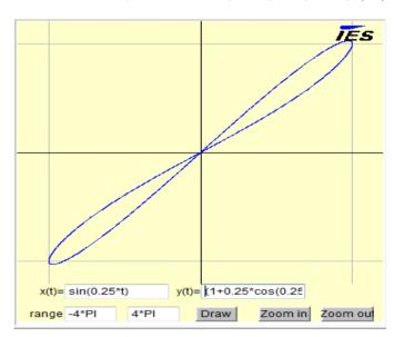
In this example the frequency was reduced to 25% of that in Example 1. The hysteresis curve begins to degenerate as the frequency is reduced and, as
