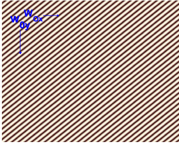
Figure 2 Computer Generated Hologram- Consists of the cosine by using Equation (5). w_{0x} and w_{0y} are determining the spacing between extrema. This relatively simple pattern of hologram provides ease, while obtaining \mathbf{f} , the object wave ( \exp[j(w_{0x}x + w_{0y}y)] ).
