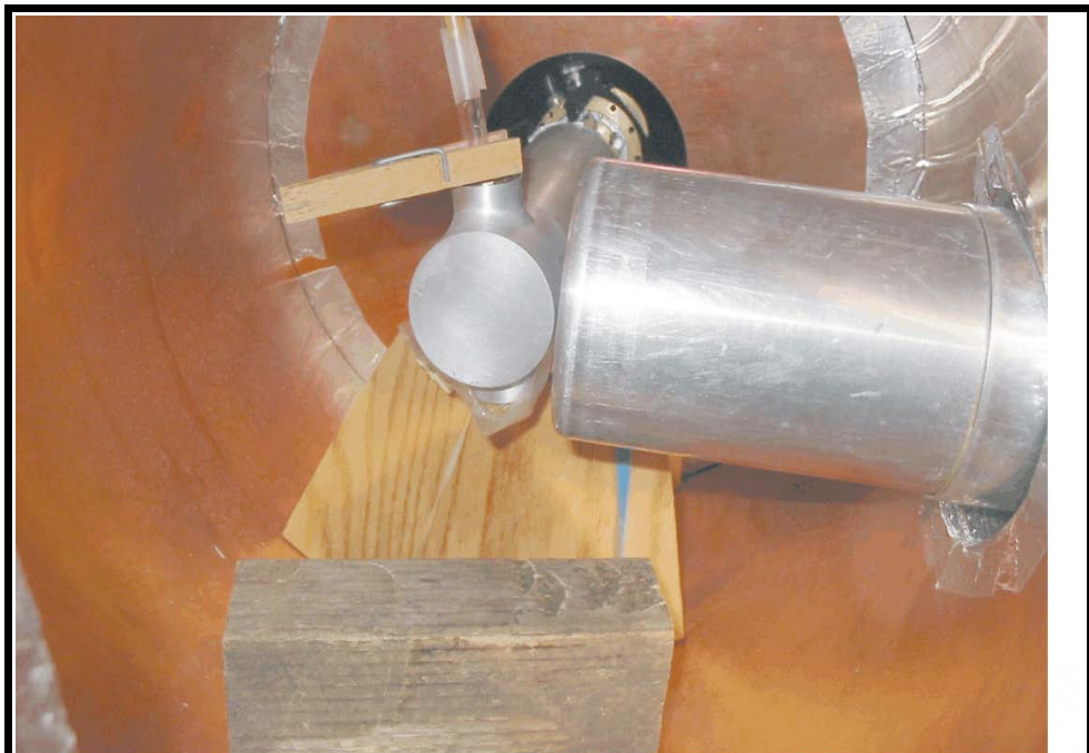
This is inside the shield. Accept for some aluminum tape, it is all lined with copper. Cd109 is in the central part of a well-hole in a 1.5 inch NaI(Tl) scintillator. HPGe is on right. Radiation must pass through the NaI to get to the HPGe. If some radiation was to scatter to the HPGe more directly, it would not matter because that is covered by the chance component we calculate and compare to. NaI generously sold by Dave Bliss. May 9, 2003. Eric Reiter.
