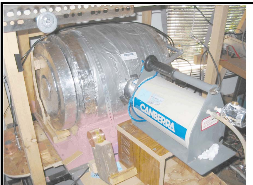
Lead shield and the HPGe (high purity germanium) detector. The HPGe was purchased from the winner of an ebay auction for $1000 without anyone knowing if it worked at all. It is reverse electrode type with a beryllium window. The lead was mostly from Allan's Steel in Redwood City. Photo of May 5, 2003. Eric Reiter
