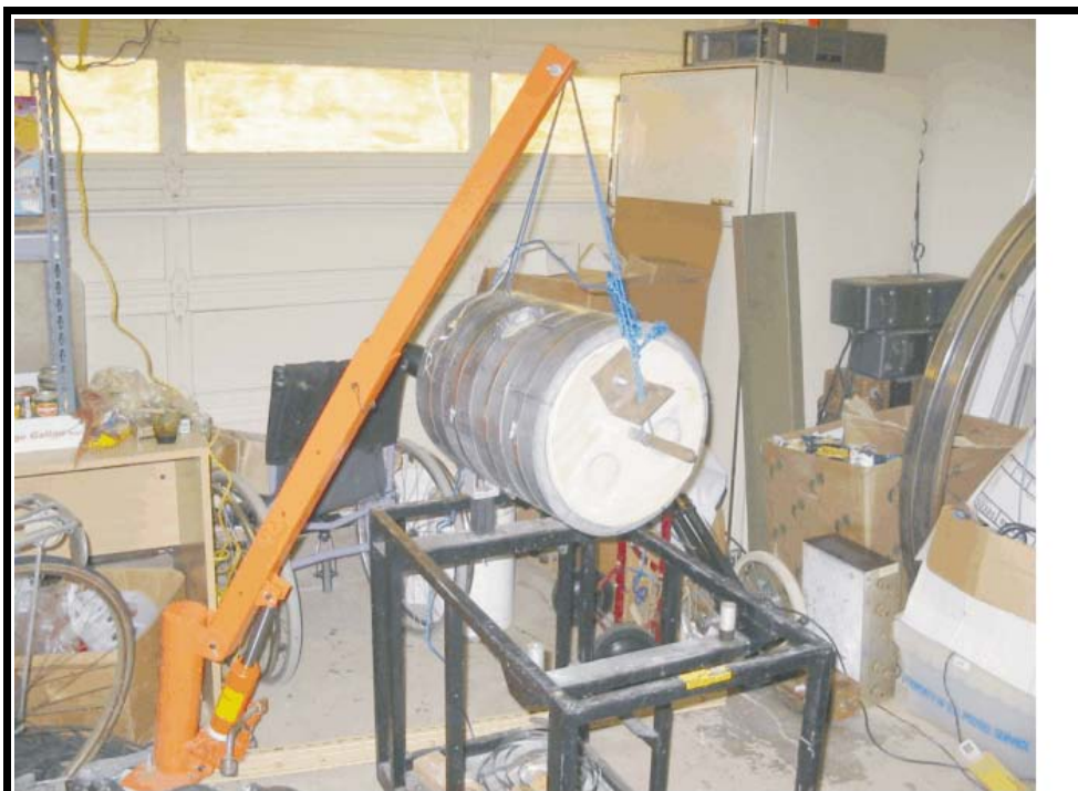
Constructing the lead shield. Bent lead bricks are strapped around a concrete mold. Shown is preparation to mount on horizontal bar for rotation on axis for further construction. Hose straps were removed. Jan 2003 Eric Reiter
