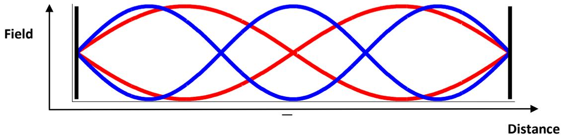
**Figure 2** , standing wave patterns in a one-dimensional enclosure
