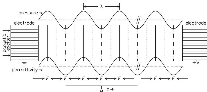
**Figure 2.** ZP energy from a standing acoustic wave in a piezo crystal. Successive close permittivity plane wave fronts introduced by an acoustic wave interact like alternating layers, giving an added Casimir force that is modulated in time with the wave oscillation.
