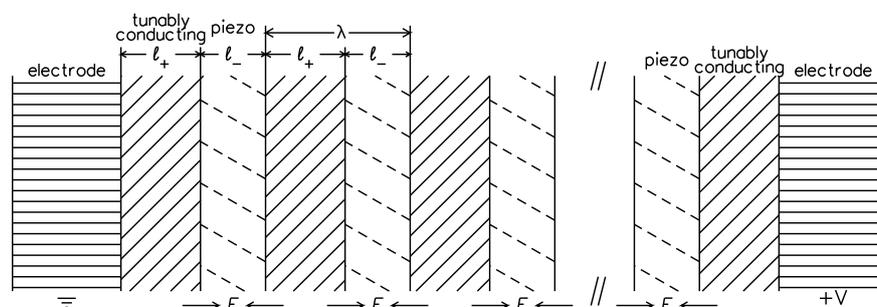
**Figure 1.** Thought Experiment: Multilayer stack of alternating tunably conductive and piezo layers. Changing the tunably conductive layers to conduct and then insulate produces a Casimir compression followed by its elastic reexpansion, which does net work on the piezo crystals from which useful electrical energy might be derived.
