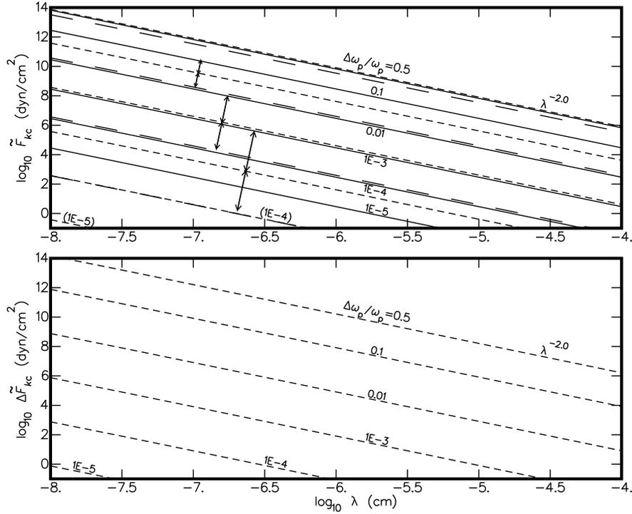
**Figure 11.** Casimir wave modes for the force  $\tilde{F}_{kc}(\lambda)$  (upper panel) and the force difference  $\Delta\tilde{F}_{kc}(\lambda)$  (lower panel) as functions of wavelength  $\lambda$  for different plasma frequency fluctuations  $\Delta\omega_p/\omega_p$  identifying wave modes as in Figure 10. A plasma frequency of  $\omega_p=1.6\text{E}16$  rad/s was used characteristic of the best normal conductors.
