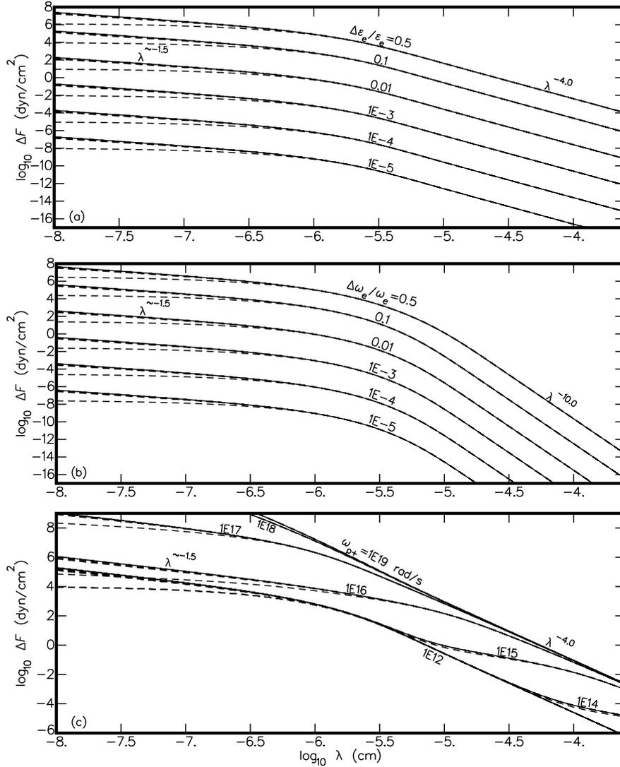
**Figure 7.** Casimir force difference  $\Delta F(\lambda)$  between normal and permittivity-reversed stacks for alternating static permittivity  $\epsilon_e$  (a), alternating electronic vibration frequency  $\omega_e$  (b), and plasma frequency in odd layers  $\omega_{p+}$  (c). Calculations with different parameter contrasts for 41 layers  $n_\ell = 20$  (solid) and fewer  $n_\ell = 1, 2, 3, 5, \dots$  (dashed) are shown.
