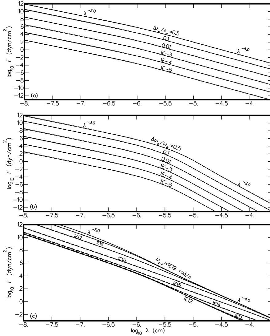
**Figure 6.** Casimir force  $F(\lambda = \ell_- + \ell\ell_+ = \ell_-/2)$  in the central layer of a multilayer stack with alternating static permittivity  $\epsilon_e$  (a), alternating electronic vibration frequency  $\omega_e$  (b), and plasma frequency in the odd layers  $\omega_{p+}$  (c). Calculations with different parameter contrasts for 41 layers  $n_\ell = 20$  (solid) and fewer  $n_\ell = 1, 2, 3, 5, \dots$  (dashed) are shown.
