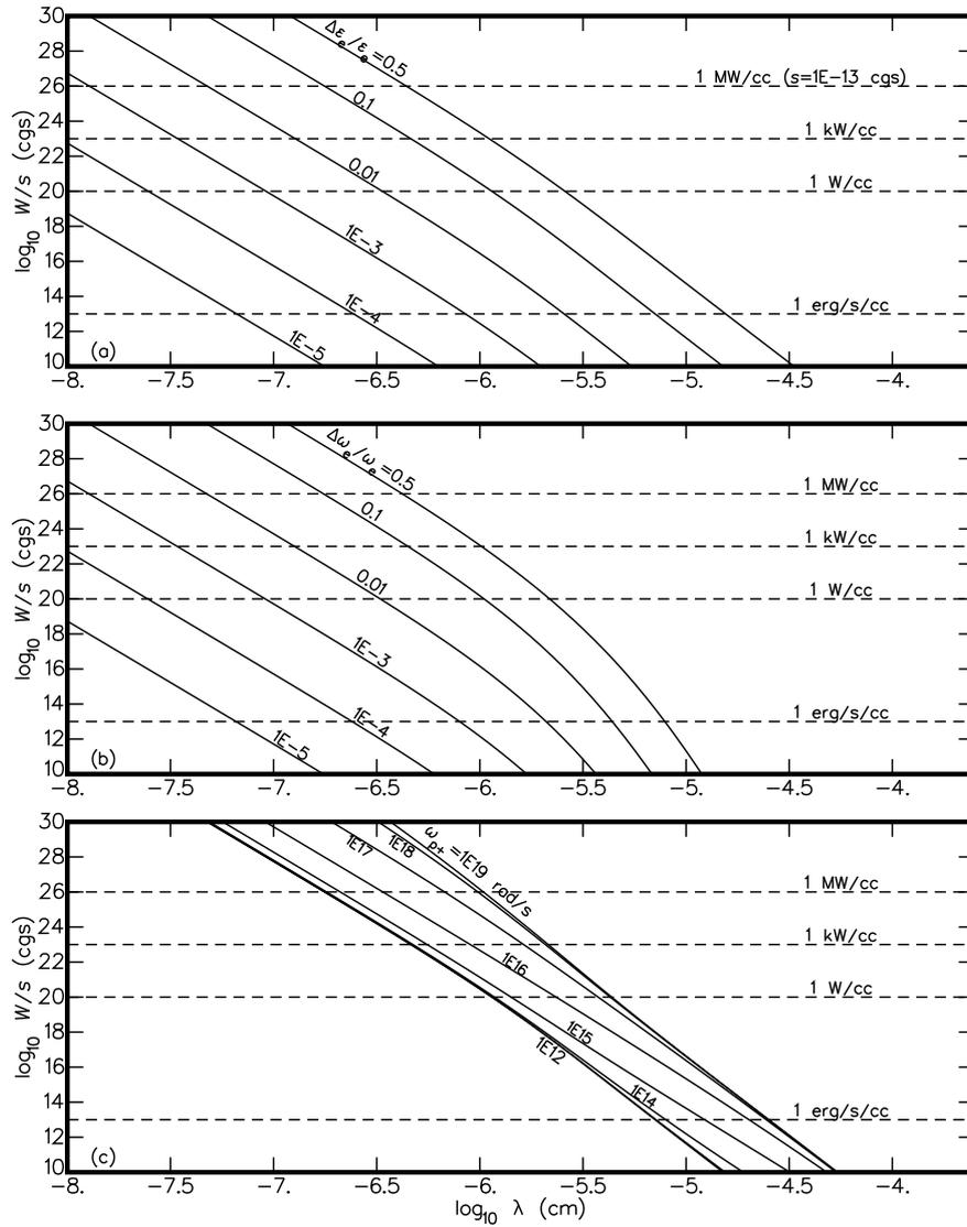
**Figure 13.** Available power per unit of crystal volume  $W$  as function of layer thickness  $\lambda = \ell_- + \ell_+$  with  $\ell_+ = \ell_-$  in a stack with alternating static permittivity (a), electronic vibration frequency (b), and plasma frequency (c) for modulation at frequencies corresponding to the sound speed  $c_s = \nu\lambda = 5E5 \text{ cm/s}$ . Horizontal power levels (*dashed*) are for material compliance  $s = 1E-13 \text{ cm}^2/\text{dyn}$ .
