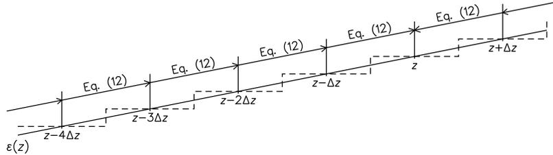
**Figure 4.** Direct calculation of Fresnel reflection coefficients in a graded-permittivity medium. A continuous permittivity variation  $\varepsilon(z)$  is approximated by discrete layers of small thickness  $\Delta z$ .
