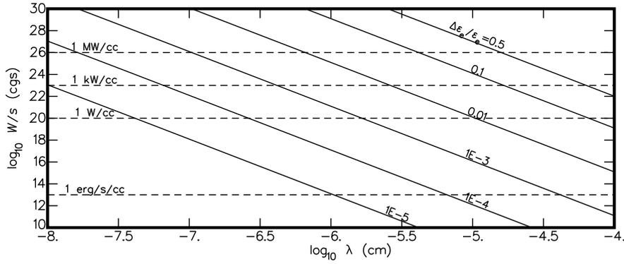
**Figure 14.** Available power per unit of crystal volume  $W$  as function of wavelength  $\lambda$  in a static-permittivity wave of indicated contrast for modulation at frequencies  $\nu$  defined by the sound speed  $c_s = \nu\lambda = 5E5$  cm/s. Horizontal power levels (*dashed*) are for a material compliance  $s = 1E-13$  cm<sup>2</sup>/dyn.
