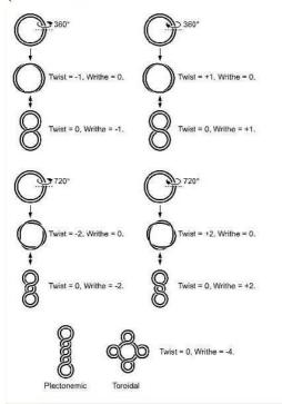
If you take a pretty long stretch, open it and add a twist (right or left) and then closes it, you'll see this spring that it distributes torque across its body in circle (second row in the image, that is positive or negative depends on the direction of the twist, ie whether left or right) (....)
