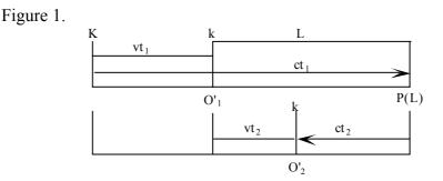
In the time  $t_1$ , the origin of **k** and the tip of the light signal should cover, respectively, the distances OO'<sub>1</sub> and OP, as shown in the upper diagram, where P(L) in Figure 1 is a fixed point in **k**. Instantaneously reflected at P, the light signal should reach the origin of **k** at O'<sub>2</sub> in the time interval  $t_2$ , as shown in the bottom of the diagram. The resulting equations
