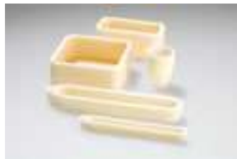
Crucible and boats made from high-temperature ceramics
